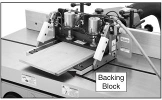
Figure 19. Backing block in place.
